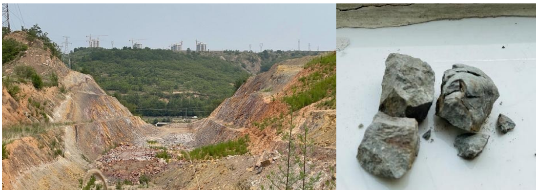
Figure 1: Raw material of gangue (Sedimentary kaolin clay) in Pingding (Yangquan) area
